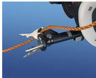
Opening the gripper traps the rope
